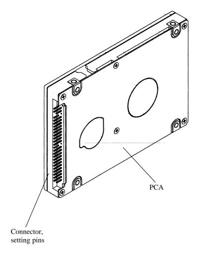
Figure 3.6 Connector locations (Sample: MHC2040AT)
